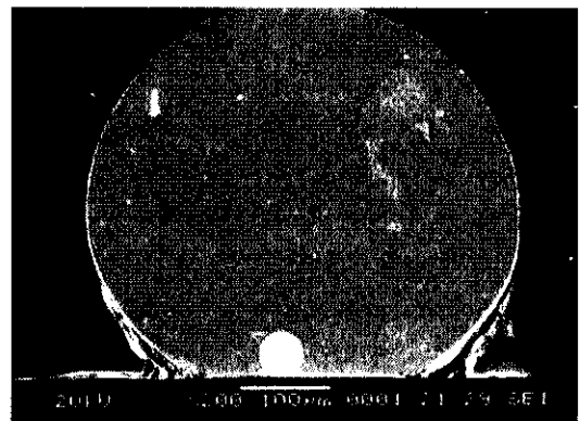
Fig. 4 Cross section of BGA solder joint showing the presence of a void
