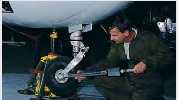
Part No TORQUE HANDLE ADJUSTABLE - DUAL SCALE 14040 Pro 650, 22mm spigot, 130 - 650 N·m, 100 - 480 lbf-ft
