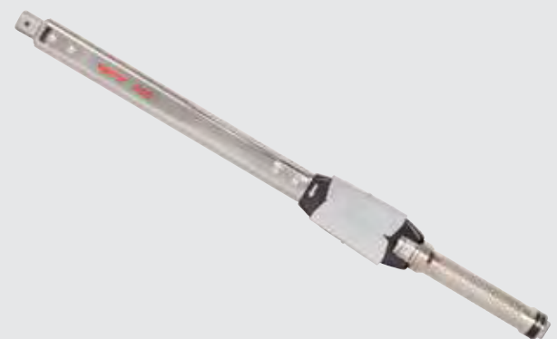
Part No FEMALE TORQUE HANDLES ADJUSTABLE - DUAL SCALE 14041 Pro 650, 14 x 18mm, 130 - 650 N·m, 100 - 480 lbf-ft
